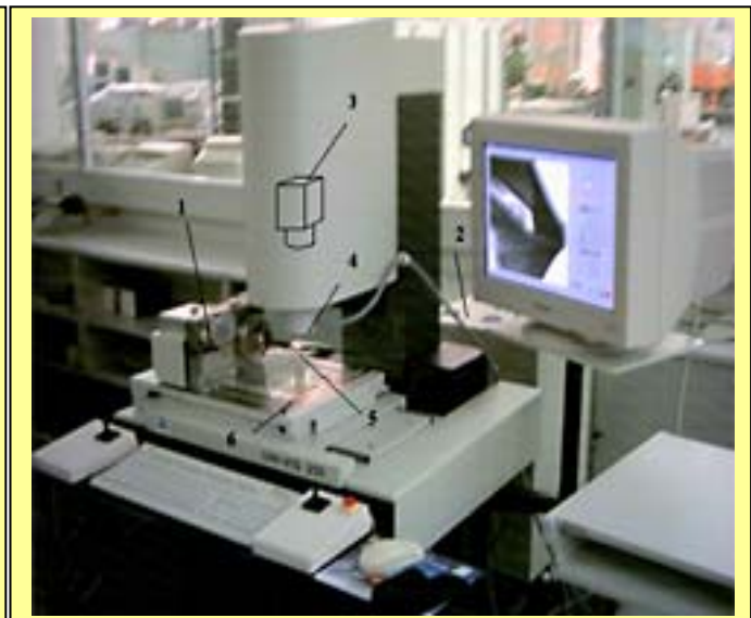
Figure 15. Optical coordinate measuring machine with twist drill [www.okm-jena.de]
