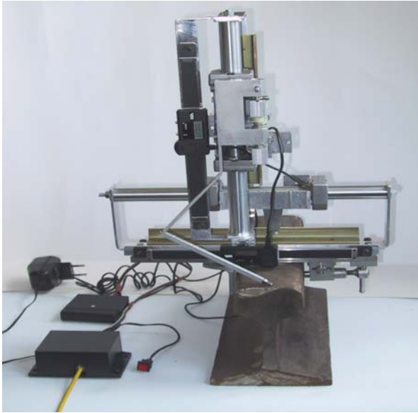
Fig. 1 A prototype device for the measurement of rails
