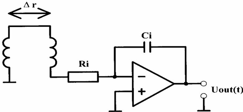
Fig.3 Apparatus for inductive measurement of magnetic field gradients
