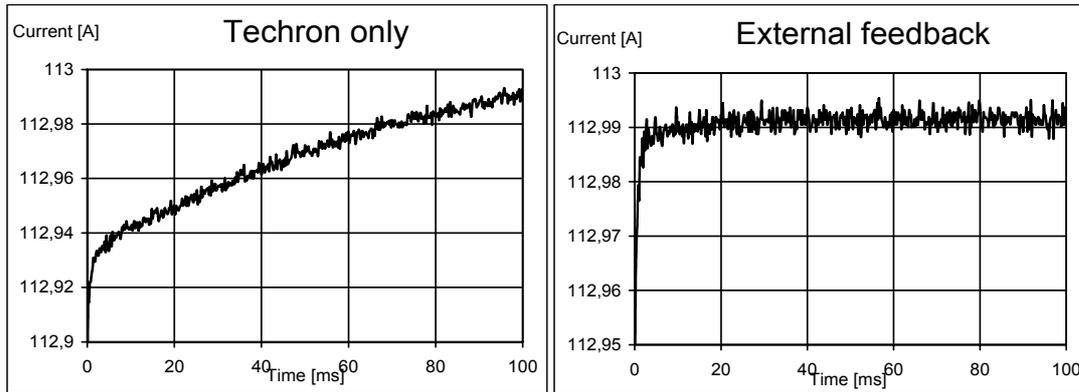
Fig.1 Output current of Techron 7780 only Fig.2 Output current with external feedback
