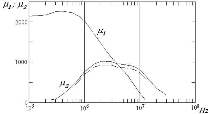
Fig.2. Magnetic spectrum for ferrite under test; — measured values; --- corrected values.
