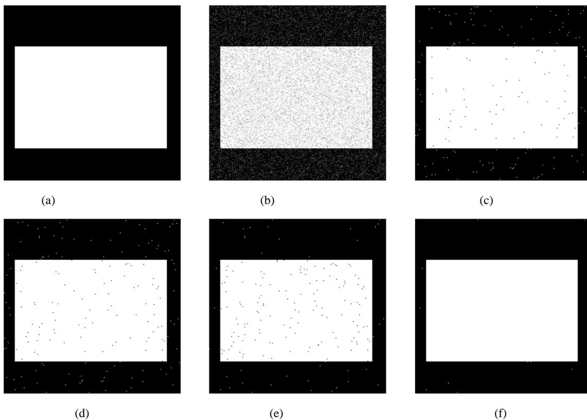
Fig.1. Results of thresholding: (a) the original image; (b) noisy image with  $SNR = 5$  ; (c) by the Jawahar's method; (d) by the Otsu's method; (e) by the Kapur's method; (f) by the proposed method.
