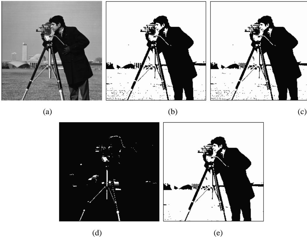
Fig.3. Results of thresholding: (a) the original image; (b) by the Jawahar's method; (c) by the Otsu's method; (d) by the Kapur's method; (e) by the proposed method.
