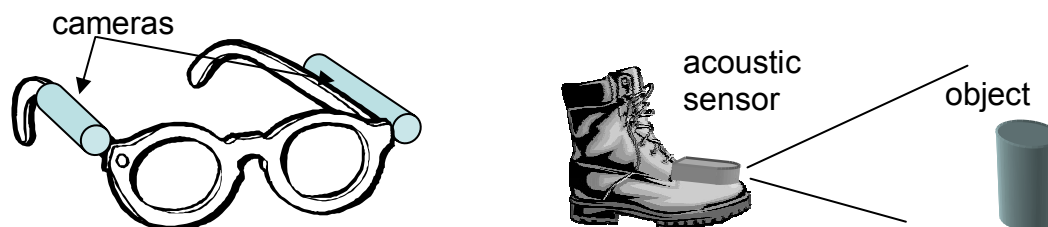
Fig. 2. Sensor systems: left: dual camera system for stereo vision, worn as glasses; right: acoustic sensor system worn on top of a shoe.
