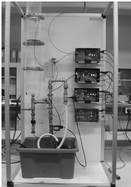
Fig. 1. Water Tower setup from the Vrije Universiteit Brussel [5]
