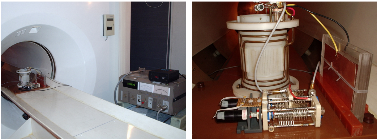
Fig. 6. Tuning control unit with the analogue RF impedance meter near the NMR image (left), detail of the matching RF coil circuit with two high quality rotating capacitors driven by special DC motors (right).
