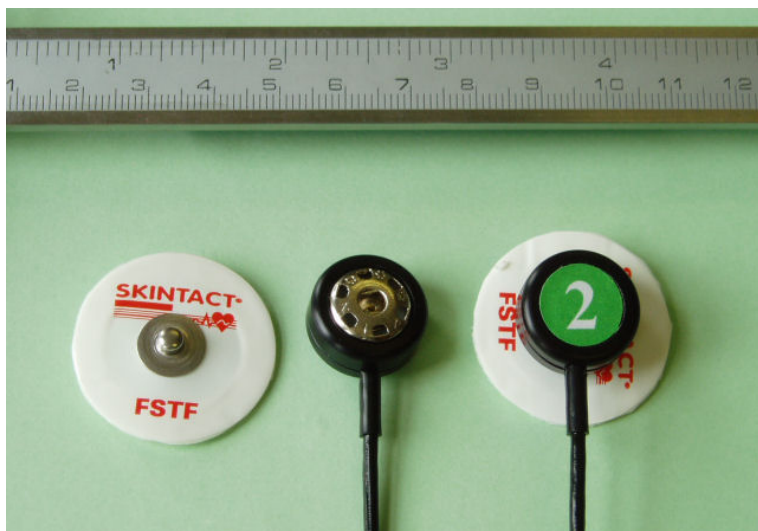
Fig. 1. Active electrodes are composed of quality Ag-AgCl disposable electrodes and active electrode adapter.
