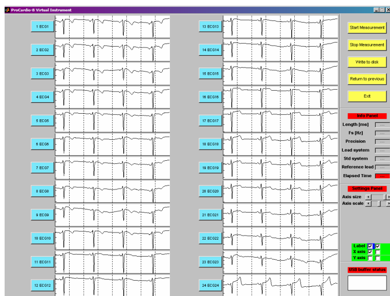
Fig. 4. Screen shot of the ProCardio 8 measurement window with monitored ECG signals from 24 leads. The contents and format of the window can be adjusted according to user requirements.
