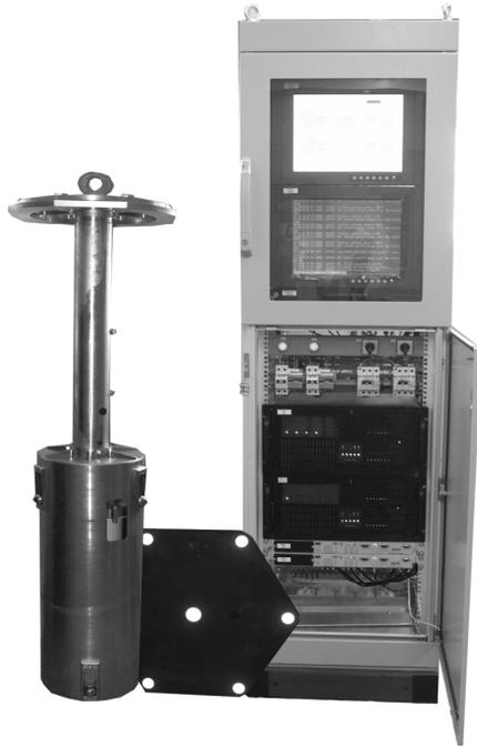
Fig. 9. System SAKHALIN: optical measuring and electronic units.
