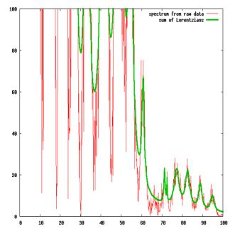
Fig.2 Raw spectrum of SR transient (thin line) and the same spectrum fitted by the weighted sum of Lorentz functions (thick line) processed in short-time (1.28 s) data set. The characteristic pattern of higher SR modes (60 - 100 Hz) is clearly visible (lower modes are out of range due to linear vertical scale). Only if the resonator is excited by a single, extraordinary intense lightning discharge, the higher modes can appear in the short-time spectra shown here.
