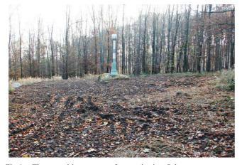
Fig.1 The capacitive antenna for monitoring Schumann resonance electric field component at AGO. The amplifier and analogue filters are placed in a small screened box directly at the bottom near the antenna base.
