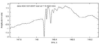
Fig.5b The same transient event recorded at Modra Observatory (AGO) also in electric field component (the time scale is different with respect to the above graph). Apparent polarity inversion of record is due to instrumental effect.
