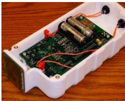
Fig.3 ICCS 2008 prototype with cover removed to show electronics (two stacked boards).
