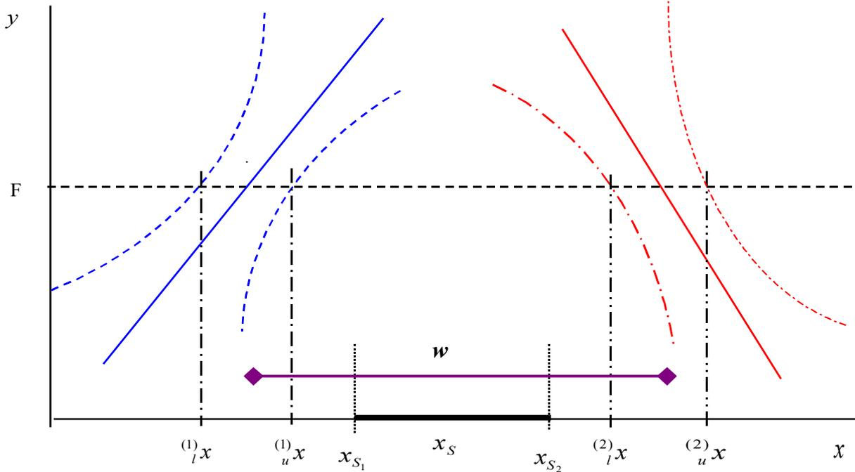
Fig.2 The confidence intervals for the structure edges  $(^{(1)}l x, ^{(1)}u x), (^{(2)}l x, ^{(2)}u x)$
