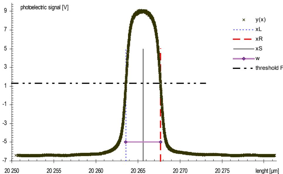
Fig.1. Photoelectric signal from a reflective microline [4].
