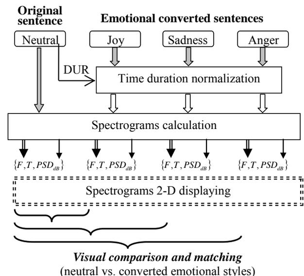
Fig.1. Block diagram of spectrogram calculation of original neutral and transformed emotional speech.
