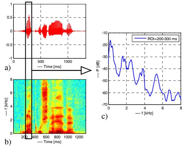
Fig.3. Example of the processed sentence “Vlak už nejede” in neutral emotional style: input signal in the time domain (a), corresponding spectrogram (b), Welch's periodogram in [dB] of selected ROI in 100-ms time interval (from 200 ms to 300 ms) (c).
