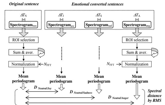
Fig.4 Block diagram of the averaged Welch's periodograms calculation and the spectral distance determination from the selected ROI areas between neutral and converted emotional styles.
