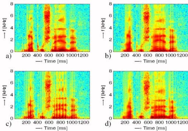
Fig.2. Spectrograms of the sentence “Vlak už nejede” (male voice,  $F_0 \approx 110$  Hz,  $f_s = 16$  kHz): original in neutral emotional style (a), resynthesis with applied normalization in the time domain – in “joyous” style (b), in “sad” style (c), and in “angry” style (d).
