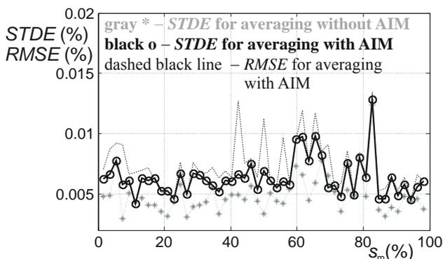
Fig. 6. STDE of ADC with averaging – STDE before and after correction by AIM compared to final RMSE.
