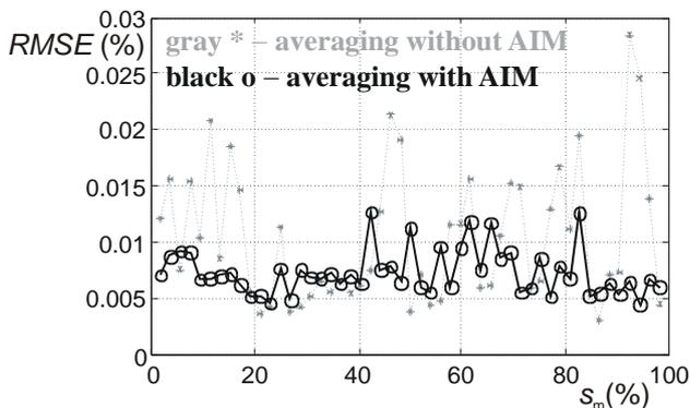
Fig. 5. RMSE of ADC with averaging before and after correction with AIM evaluated in each point of range for quasi-optimal standard deviation of dither.
