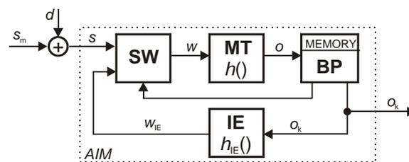
Fig.1. Block diagram of our measuring system, the part in frame corresponds to AIM.
