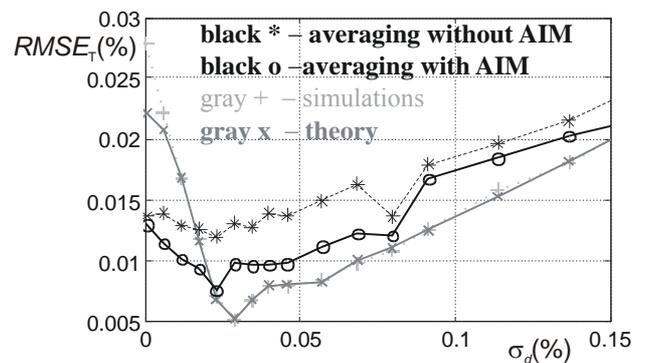
Fig.4. Total RMSE of ADC with averaging before and after correction with AIM.
