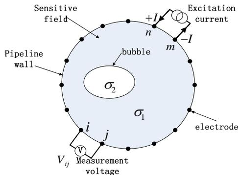
Fig.1. Schematic diagram of ERT sensor
