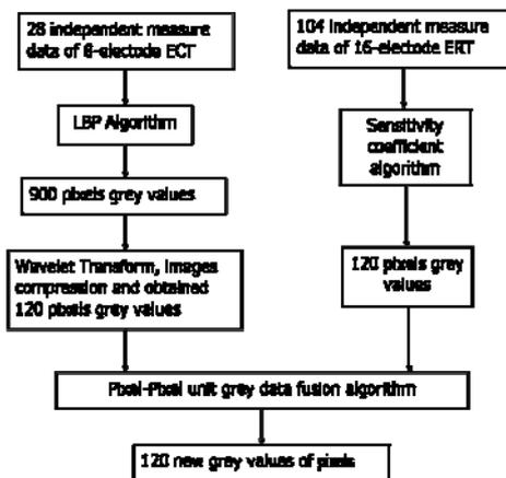
Fig.7. The diagram of data fusion process
