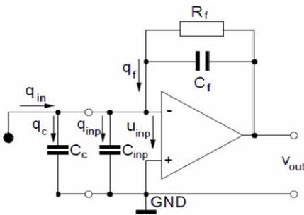
Fig.11. The diagram of charge amplifier
