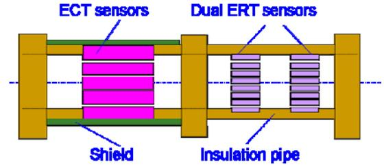
Fig.4. Fusion sensor of ECT sensors with dual ERT sensors
