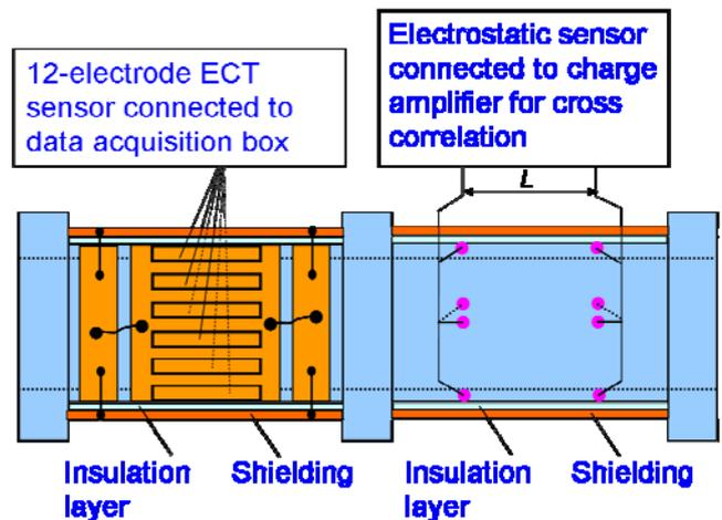
Fig.9. The diagram of ECT and electrostatic sensors
