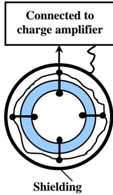
Fig.10. The section diagram of electrostatic sensor
