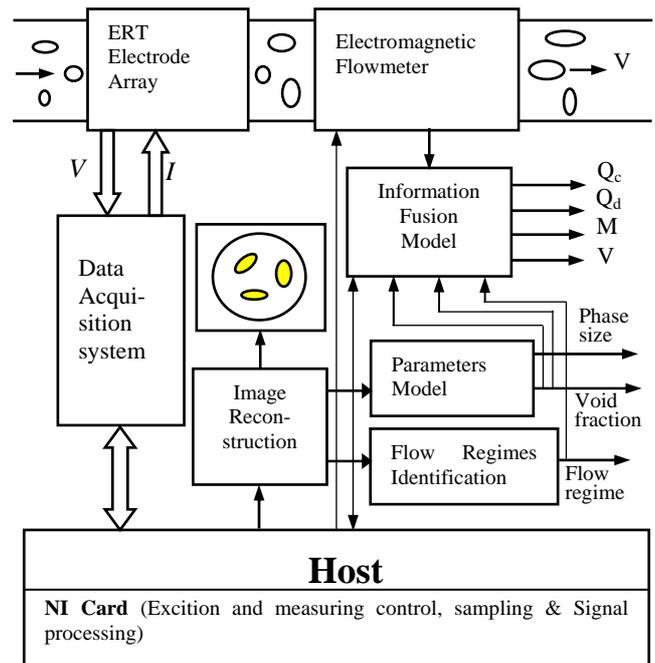
Fig.2. The diagram of the whole measuring system
