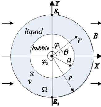
Fig.3. The electrodes section diagram of EM flow-meter
