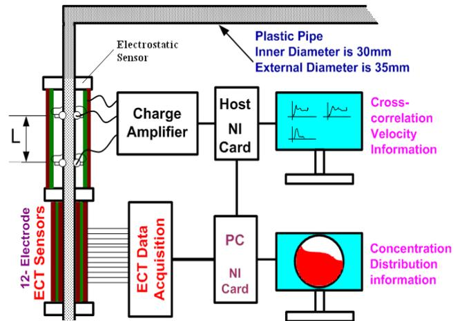
Fig.8. The fusion system of ECT with Electrostatic sensors
