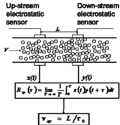
Fig.13. The diagram of correlation operation
