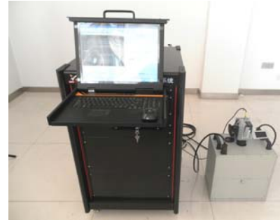
Fig.1. The pulsed heating infrared thermal wave non-destructive test system
