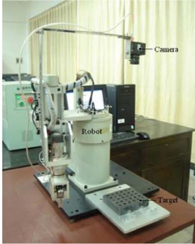
Fig.5. Vision system and manipulator
