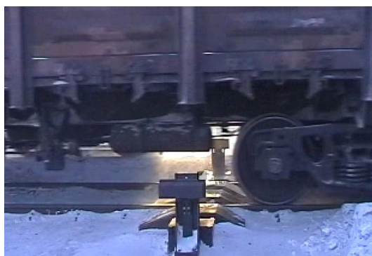
Fig.8. Laser diagnostic system COMPLEX for wheel pair inspection operating in winter conditions at the West-Siberian Railway.
