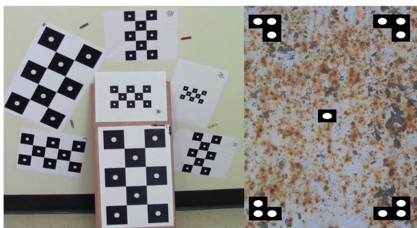
Fig.2. The multi-resolution, multi-depth test-field for camera calibration test-field (left) and the object pattern designed from rusted metal texture and circular evaluation marks (right).
