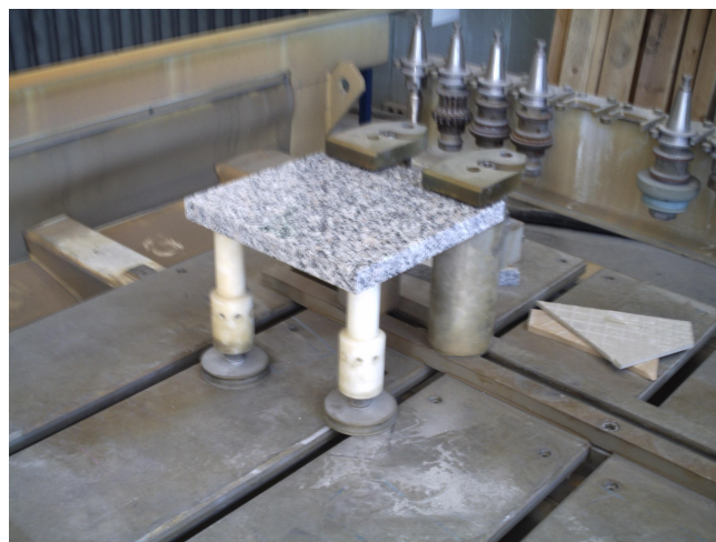
Fig.6. Fixing the granite block in the NC machine-tool.
