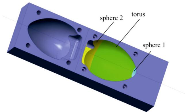
Fig.1. Complex workpiece surface separated into geometric features.
