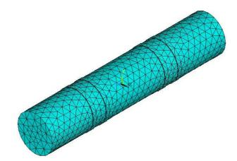
Fig.7. The meshed 3D model of the RSCP with 10692 elements:  $L_e = 0.10 \text{ m}, D = 0.02 \text{ m}, h_e = 0.002 \text{ m}, h_m = 0.002 \text{ m}, S_e = 0.047 \text{ m},$  $S_m = 0.032 \text{ m}, \sigma_w = 100 \Omega \text{m}.$
