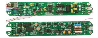
Fig.13. Images of frequency measurement circuitry for the SGLCP and RSCP.
