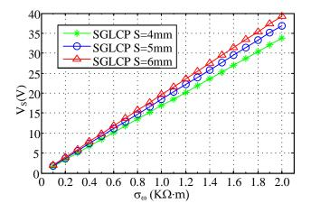
Fig.10. Calculated response of the simulation for the SGLCP under different values of  $\sigma_w$ : h=2 mm, d=1.5 mm, D=20 mm.
