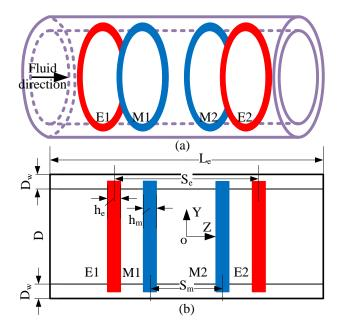
Fig.3. Geometry and parameter definition of the RSCP: a) 3D model; b) 2D structure.
