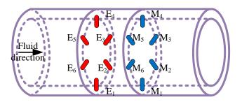
Fig.1. Geometry of the SGLCP for dynamic pure-water measurement.
