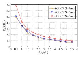
Fig.17. Calibration of the SGLCP under different values of  $\rho_w$ : h=2 mm, d=1.5 mm, S=4, 5, 6 mm, respectively.
