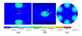
Fig.6. Electric field distribution of the SGLCP: a) YoZ plane section view; b) XoZ plane section view; c) XoY plane section view.
