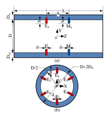
Fig.2. Sketches of structure parameters and coordinates of the SGLCP: a) The axial section; b) The cross section.
