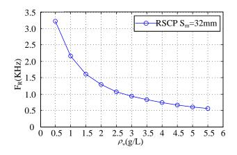
Fig.18. Calibration of the RSCP under different values of  $\rho_w$ :  $h_e = 2$  mm,  $h_m = 2$  mm,  $S_e = 47$  mm, c=32 mm.
