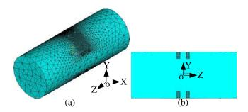
Fig.4. The meshed 3D model of the SGLCP with 250295 elements: L=0.05 m, D=0.02 m, h=0.002 m, d=0.0015 m, S=0.004 m, water resistivity  $\sigma_w = 100 \ \Omega m$ : a) 3D model; b) The axial section.
