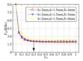
Fig.16. Calibration of the LCP<sub>1</sub> with  $\rho_w = 2.0 \text{ g/L}$  under different  $y_m$  in the condition of oil-water segregated flow.
