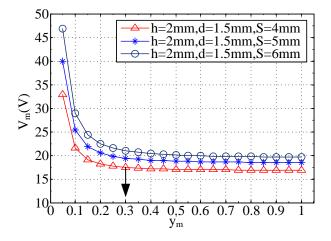
Fig.9. Calculated response of the simulation for LCP<sub>1</sub> under different values of  $y_m$ : D=20 mm,  $\sigma_w = 100\Omega m$  and oil resistivity  $\sigma_o = 1.0E + 13\Omega m$ .
