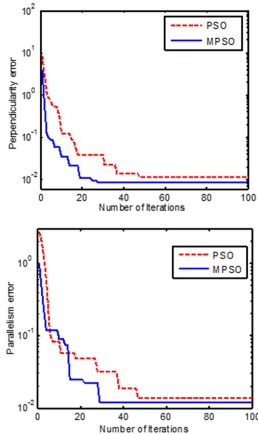
Fig.7. PSO and MPSO algorithm for perpendicularity and parallelism error.
