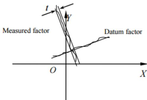
Fig.1. Schematic for determining perpendicularity.
