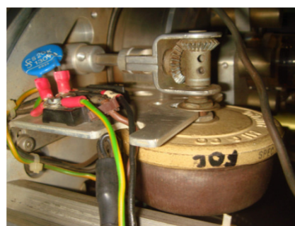
Fig. 4. Gear and potentiometer that controls the focusing voltage supply.
