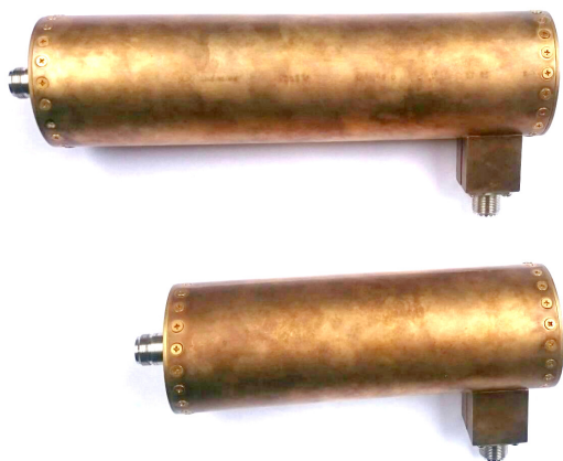
Fig.2. Two primary calculable AC Voltage Standards developed at SUT.
