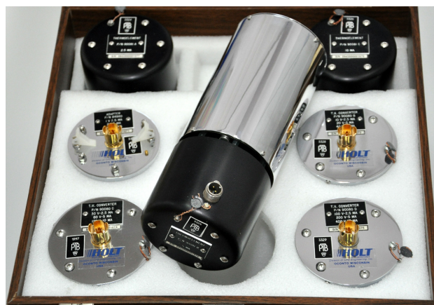
Fig.1. A set of AC Voltage Standards (Holt model 11) maintained by GUM with the SJTC on the top. Range resistors are inserted into box slots.
