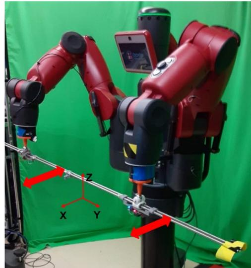
Fig.7. Experimental settings of the Baxter robot with the proposed motion gauge attached; the coordinate frame and the linear motion indicated by the red arrows.
