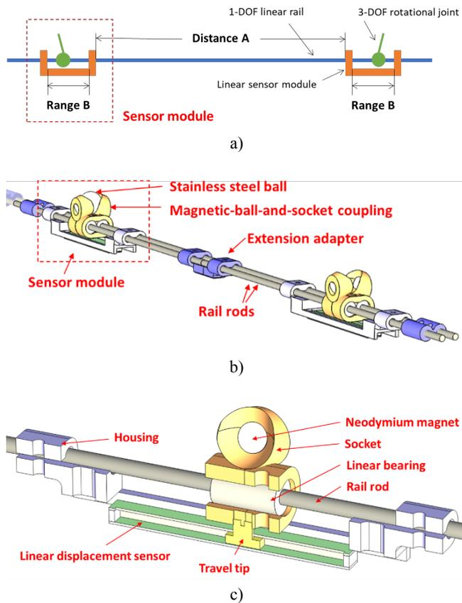
Fig.2. Designs of the proposed motion gauge system: a) a conceptual design, b) a full 3D CAD model; and c) a cross-sectional view of the sensor module.
