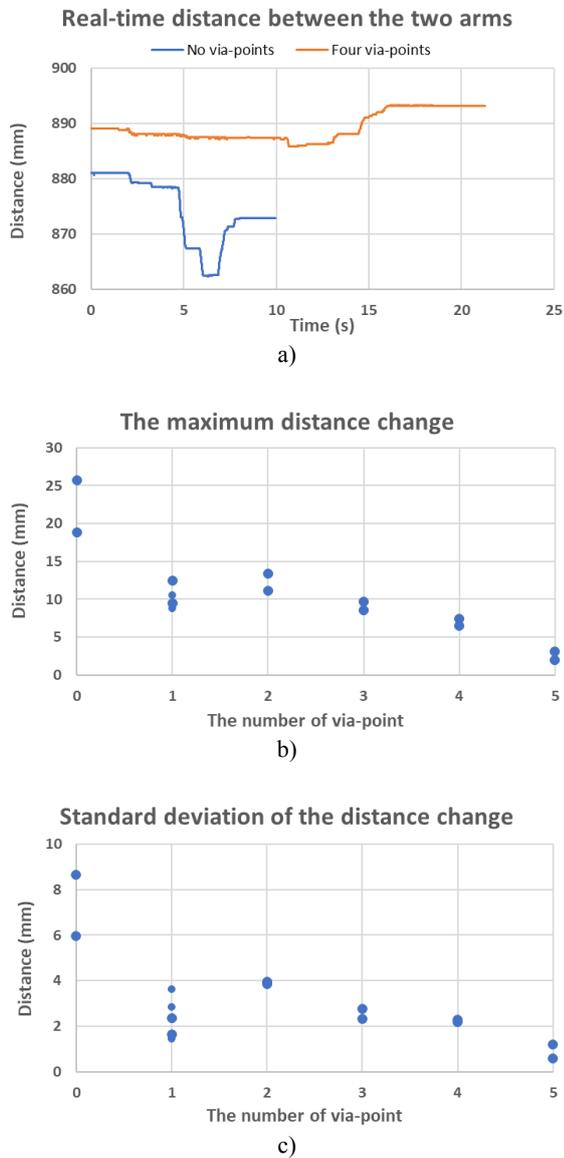
Fig.8. Distance between the two arms of a robot as measured by the proposed metrology bar gauge: a) real-time distance between the two arms, b) the maximum distance change as a function of the number of via-points, and c) the standard deviation of the distance change as a function of the number of via-points.
