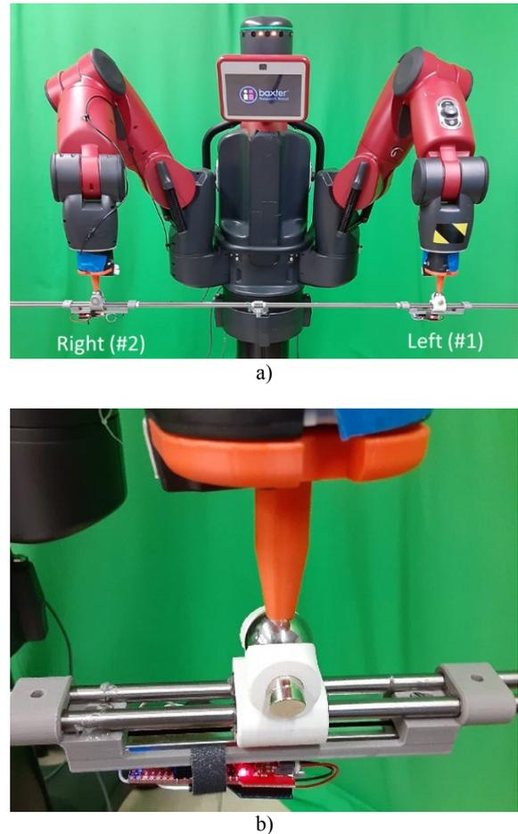
Fig.5. The fabricated Wireless Motion Gauge system: a) installed on two arms of a Baxter robot, b) the sensor module.
