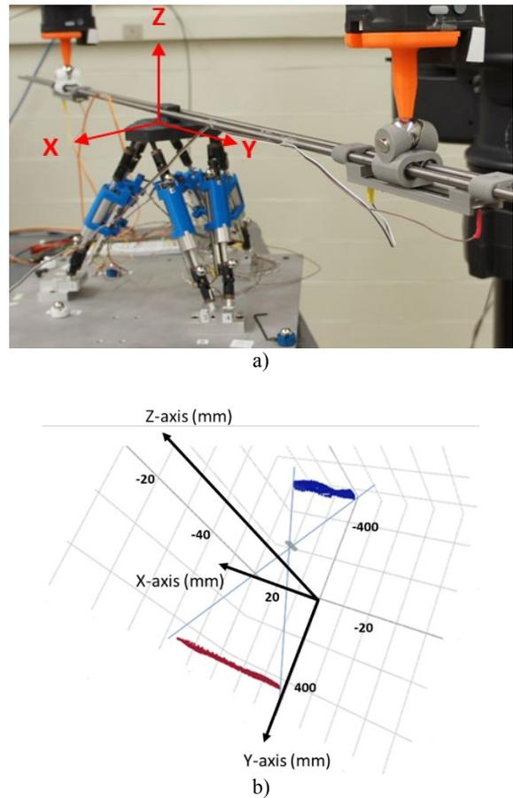
Fig.9. The metrology bar gauge mounted on an independent 6-DOF metrology system: a) The 6-DOF metrology system is based on a Hexapod Stewart platform; b) Measurement of the 3D positions of the two robot arms, while they are programmed to simulate the motions of turning a circular valve handle.
