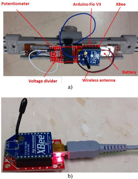
Fig.4. The sensor module: a) the sensor module with the wireless signal conditioning unit, and b) the wireless receiver module connected to a remote computer.
