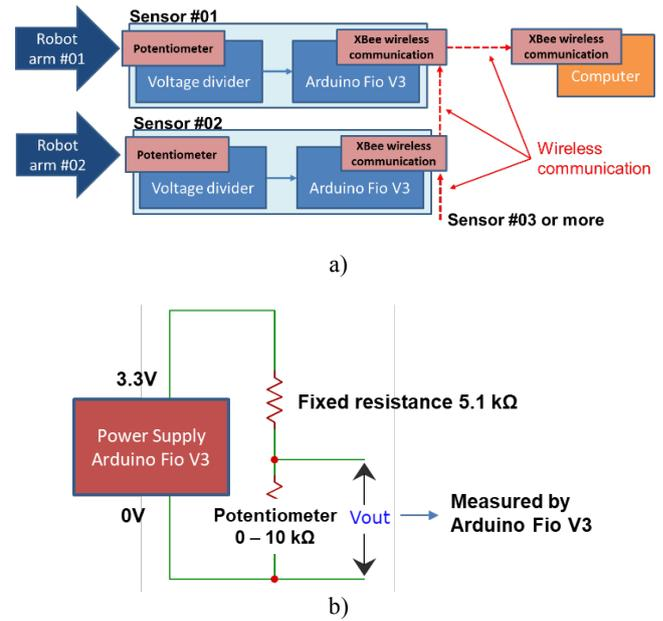
Fig.3. The wireless signal conditioning unit: a) the wireless connection diagram, and b) the voltage divider.
