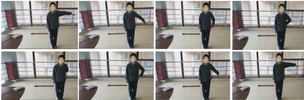
Fig.7. Skeleton point occlusion test of arm swing (unfold-occlusion-unfold).
