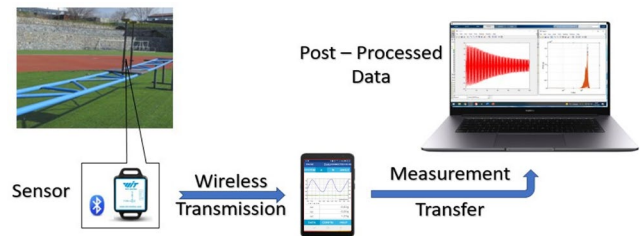
Fig. 3. Wireless accelerometer system configuration.
