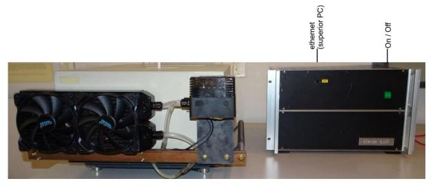
Fig. 4. Benchmark from the front. The NMR sample cooling device is mounted on a permanent magnet housing.
