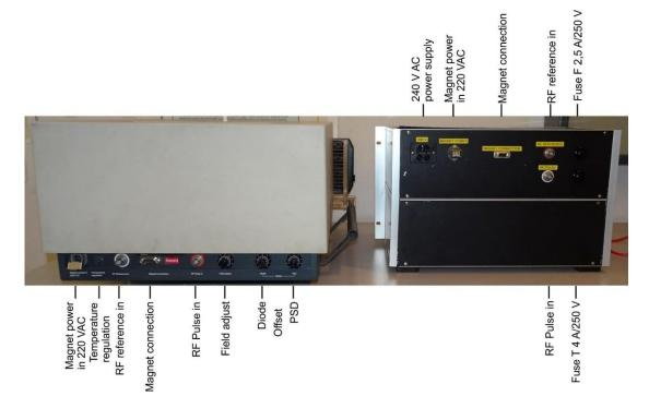
Fig. 5. Benchmark from behind. Here is the vast majority of connectors and some controls. The corresponding connectors must be connected by dedicated cables.
