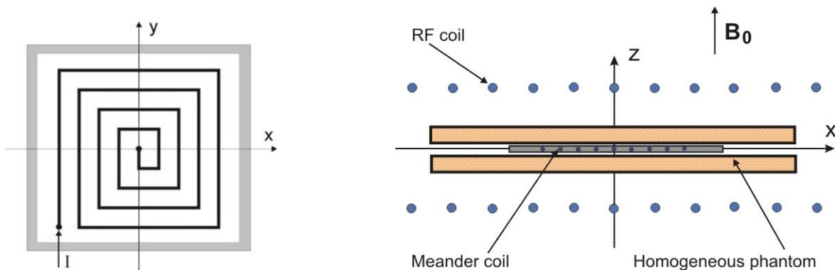
Fig. 3. Left: Meander planar coil design, dimensions 60 x 60 mm, realized on a printed board. Right: RF coil, active measuring volume (homogeneous phantom) and meander planar coil.
