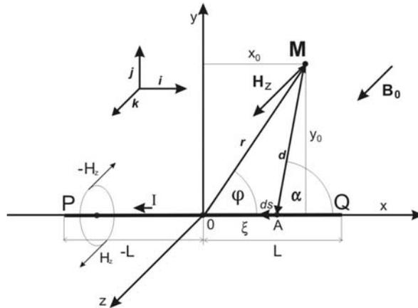
Fig. 1. Basic configuration of the limited length conductor  $\overline{PQ}$  placed into the  $x$  – axis.
