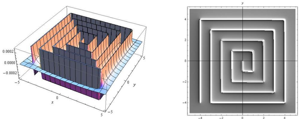
Fig. 2. Calculated magnetic field  $H_z(x,y)$  of the planar meander rectangular coil, limited plot-range. Left: 3D-plot of relative values. Right: Density-plot of relative values.
