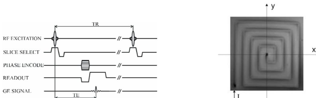
Fig. 4. Left: Time diagram of the NMR sequence for the gradient-echo signal detection. TE - echo time of 18 ms, TR – repetition time of 300 ms. Right: NMR image of the magnetic field distribution of a meander planar coil (60 x 60 mm), number of measured voxels 150 x 150.
