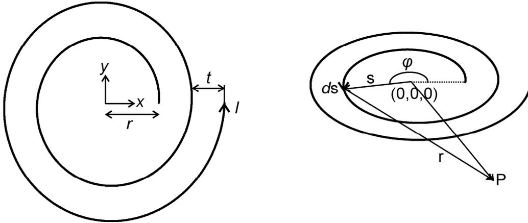
Fig. 1 Two-turn spiral-shaped coil.
