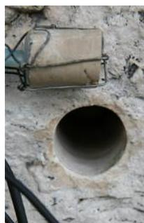
Fig. 5. The moisture sensor and hole configuration.
