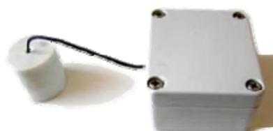
Fig. 3. The RTM 1.01 instrument in connection with the hot ball arranged as a moisture sensor.
