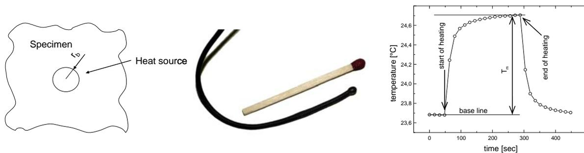
Fig. 1. Model of the hot ball and its realization (left). Measuring cycle measured at sandstone for hot ball heat output  $q = 3.5$  mW (right).
