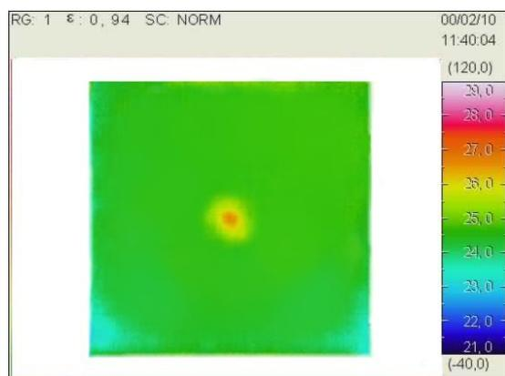
Fig.6 Thermogram of the object under test with subsurface defect in the middle
