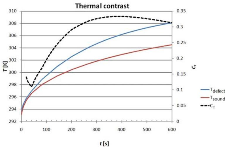
Fig.5 Time dependence of the thermal contrast between defect and sound area
