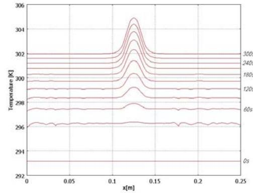
Fig. 4 Time evolution of the temperature along the surface line of the object with subsurface defect irradiated by IR radiation – results from FEM model
