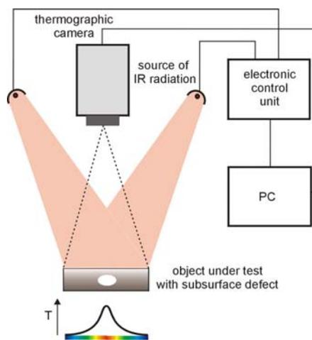
Fig.1 Basic set-up of active infrared thermography
