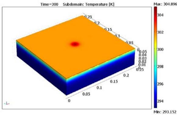
Fig. 3 Temperature field of the object with subsurface defect irradiated by IR radiation – pseudo-colour presentation of FEM model results
