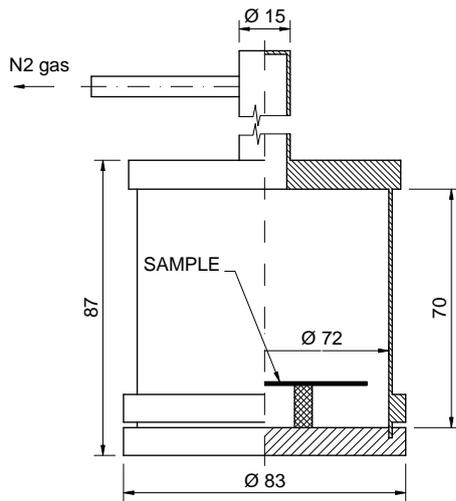
Fig. 1. The sketch of the calorimeter.
