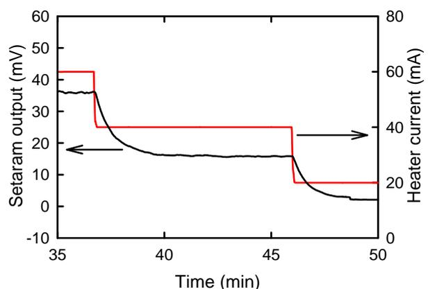
Fig. 4. The dependence of  $V_f$  on time recorded during the change of the heating current  $I_h$  from 60 mA to 40 mA and from 40 mA to 20 mA.
