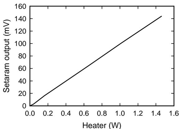
Fig. 3. The calibration curve of the calorimeter. The calibration constant is  $K_c = 98.84$  mV/W.
