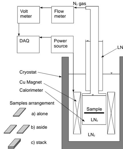
Fig. 2. Schematic view of experimental set-up and samples arrangement in the calorimeter.
