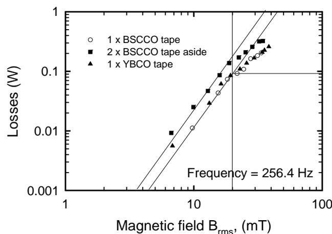
Fig. 6. The AC losses of one and two pieces of BSCCO tape 50 mm long. Also losses of 4 mm wide YBCO tape are shown for comparison.
