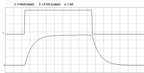
Fig. 5: Response to 10 mV input step
