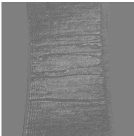
Fig. 2. The picture of discharge gap at the applied voltage 1.2 kV and gap distance 0.4 mm.
