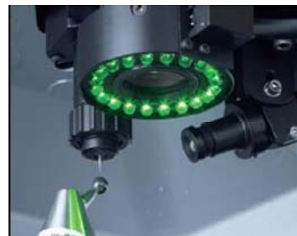
Deployed multi-sensor coordinate measuring machine (on the left), the orientation of the machine coordinate system (in the middle), probing sensors of the MS-CMM (on the right) [1]
