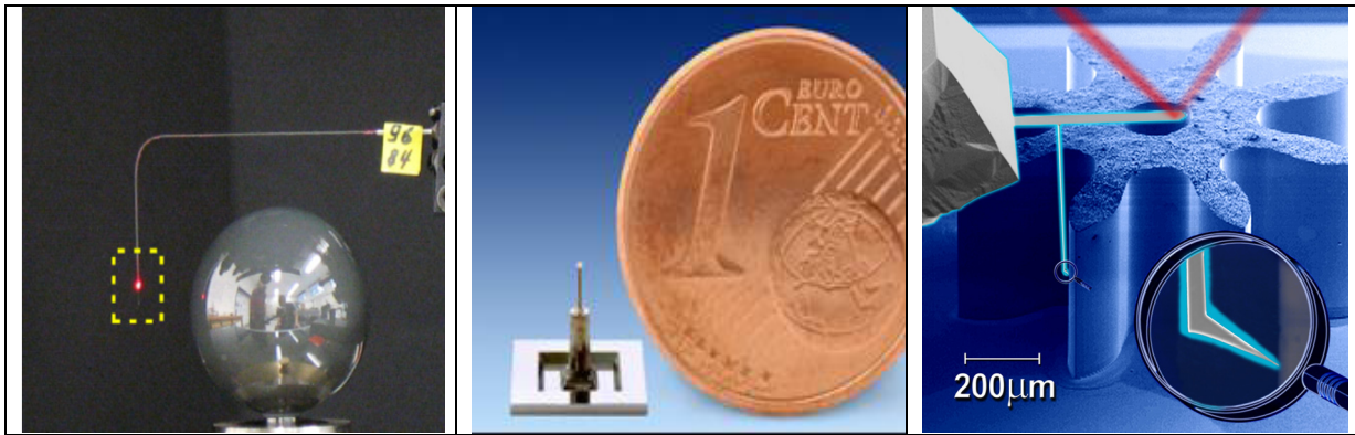
Fig 2. Microprobe systems developed and used at the PTB for characterization of microcomponents. Left: opto-tactile 3D probe; middle: Si boss membrane 3D microprobe (with Euro Cent coin for size comparison); right: ACP probe (assembled cantilever probe).
