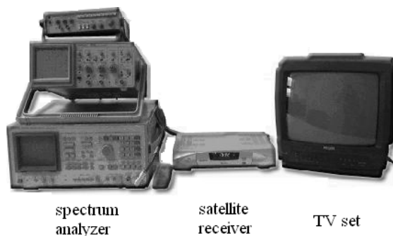
Fig. 2. Setup realisation for measuring the satellite signal.
