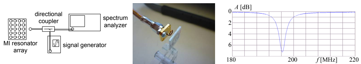
Fig. 1. Setup for resonant curve of single resonator measurement (left), the loop probe detail (middle) and an example of measured characteristic (right).
