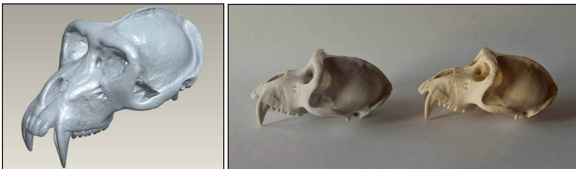
Fig. 1. STL model of monkey skull generated from point cloud (left) and copy of skull made with rapid prototyping technology compared to real skull (right)
