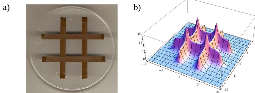
Fig. 4. a) Original sample made of 4 low magnetic tapes, double cross, 6 x 70 mm, distance between tapes 25 mm, audio cassette tape, thickness 11  $\mu\text{m}$ , densely packed pure grained ferric particles. b) Calculated 3D image of the magnetic field distribution.
