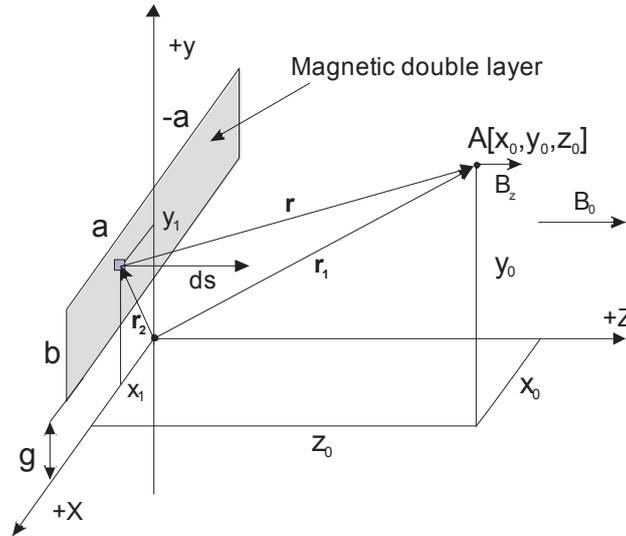
Fig. 1. Basic configuration of the magnetic double layer sample positioned in x-y plane of the rectangular coordinate system. The thickness of the layer is neglected.
