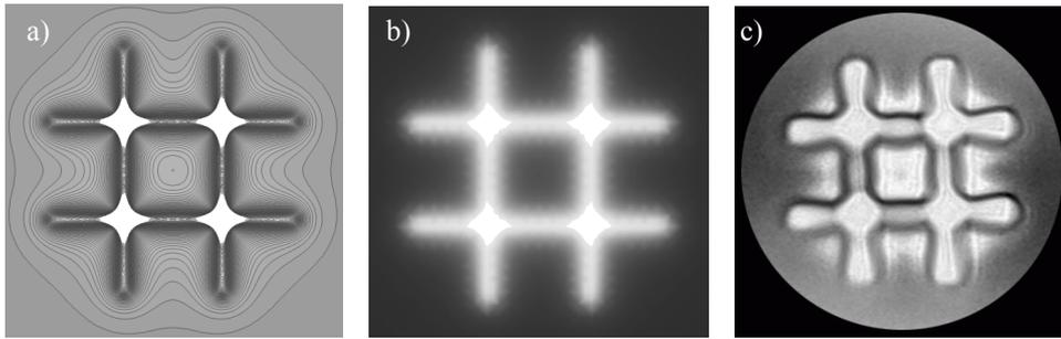
Fig. 5. a) Calculated image of the magnetic field, contour plot, b) density plot, c) NMR image of the double cross sample using GRE imaging sequence.
