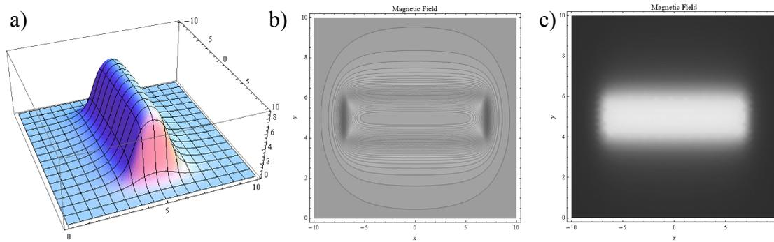
Fig. 2. Calculated magnetic field  $B_z(x,y,z)$  of the magnetic double layer sample positioned in x-y plane of the rectangular coordinate system. a) 3D-plot, b) contour plot, c) density plot.
