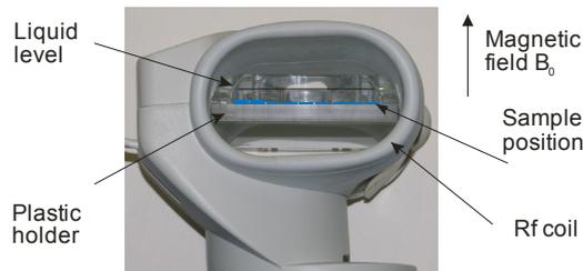
Fig. 3. Horizontal field RF coil, active measuring volume (homogeneous phantom), dimensions 90 x 90 mm.
