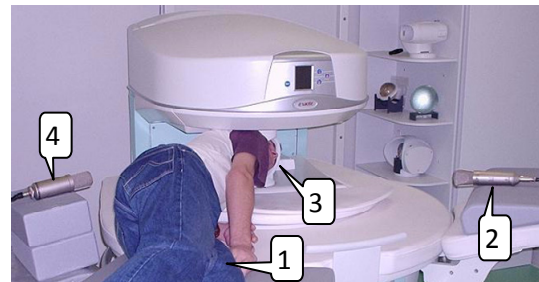
Fig. 3. An experiment arrangement: bed with testing person (1), front read microphone 1 (2), patient's head into RF coil (3), back read microphone 2 (4).
