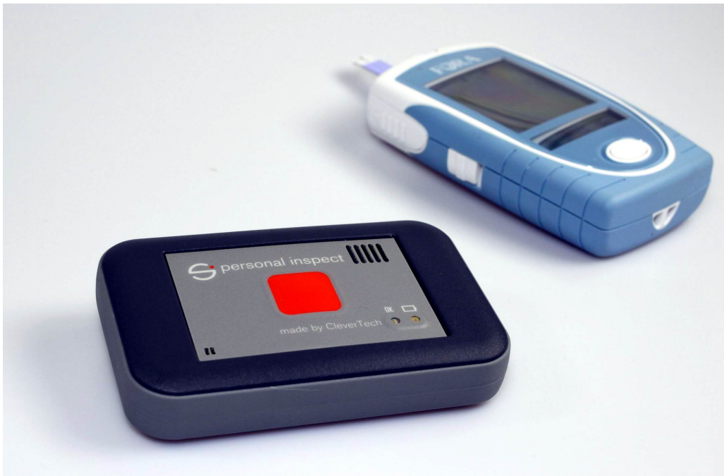
Fig. 1. Personal inspect mobile sensing unit (left) with wirelessly connected blood glucose meter (right).
