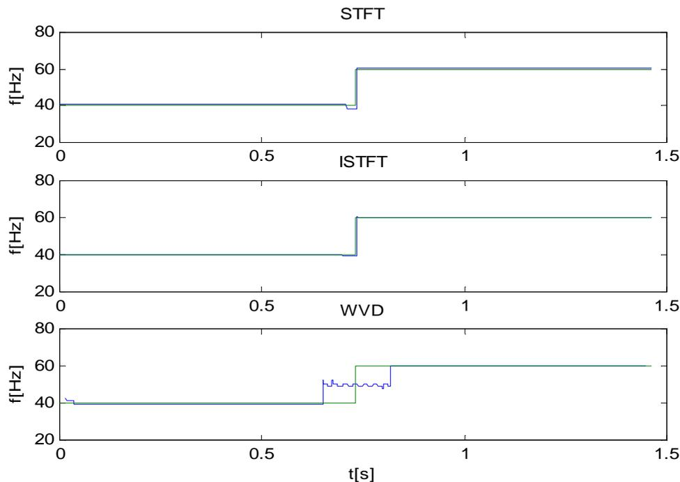
Fig.1 An abrupt change in signal frequency from 40 Hz to 60 Hz and corresponding outputs of instantaneous frequency gained by STFT, interpolated STFT and by WVD
