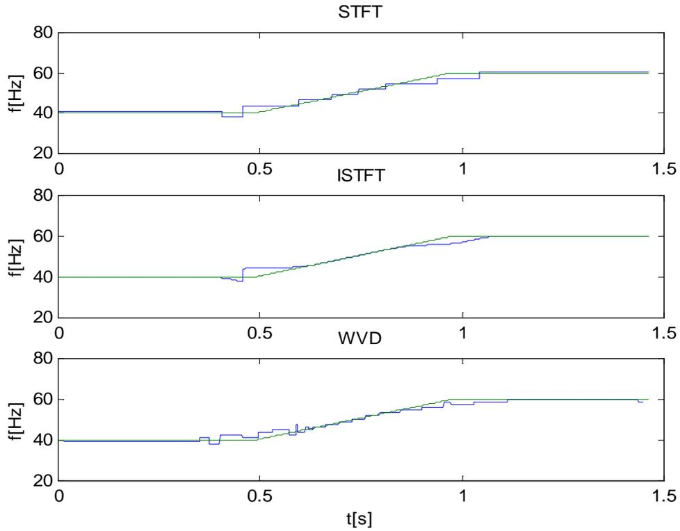
Fig.2 Linear change in signal frequency from 40 Hz to 60 Hz and corresponding outputs of instantaneous frequency gained by STFT, interpolated STFT and by WVD.
