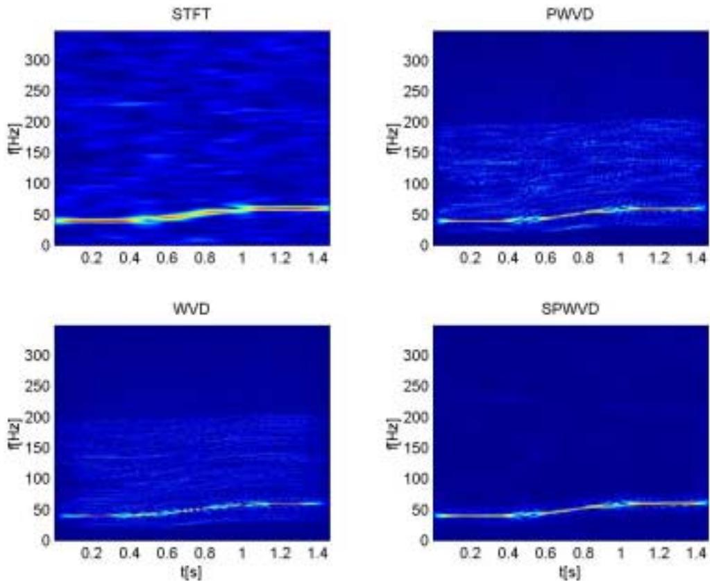
Fig.3 Time-frequency signal representations gained for the sinusoidal signal with frequency change according to Fig.2. Signal is mixed with additive white Gaussian noise, SNR=0 dB.
