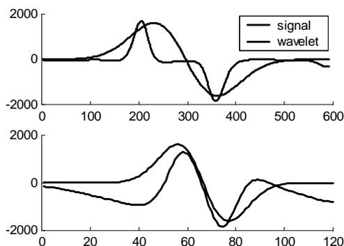
Figure 2. Correspondence between Gaussian wavelet and typical signal of indications (support plate, defect-hole)
