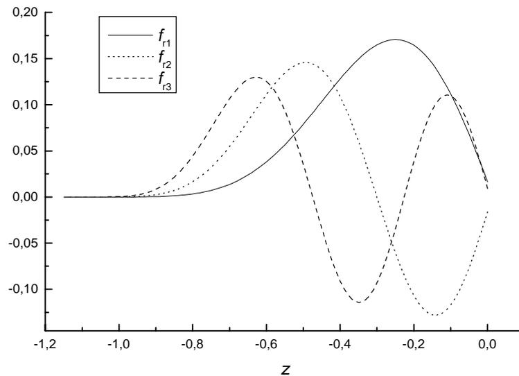
**Fig. 9.**  $H_{01}$  amplitudes of the first, second and third resonance in GTEM-cell
