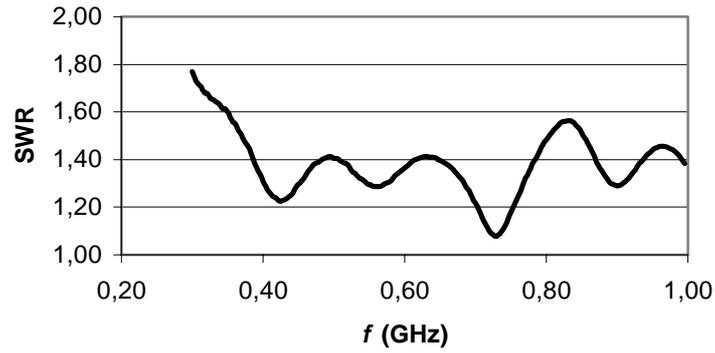
**Fig. 6.** SWR of GTEM-cell up to 1GHz
