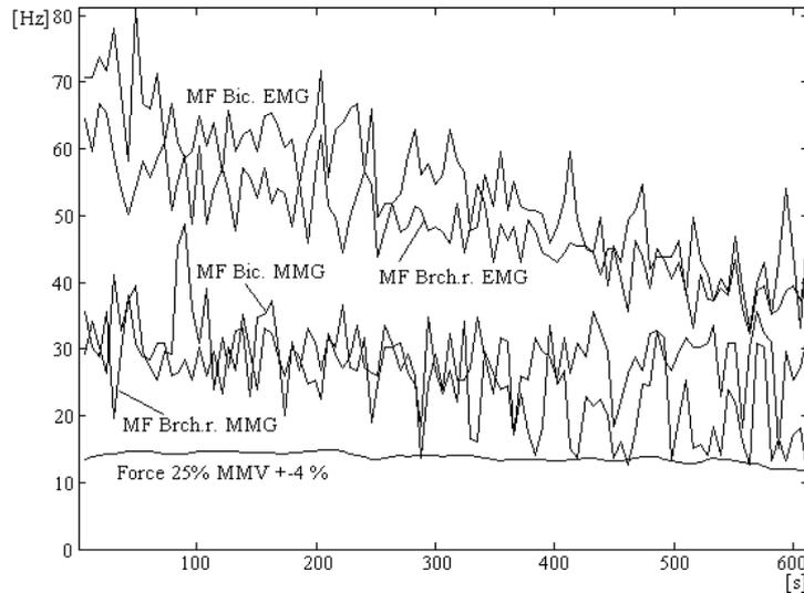
**Figure 2.** The evolution of the MF of the EMG and MMG signals for one subject. The force, averaged on each buffer slightly oscillates around 25% MVC. MF decreases from the very beginning of the exercise, both for the EMG and MMG, for the both muscles involved.
