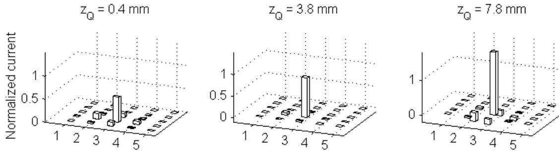
Fig. 3. The normalized currents on the anodes when charge  $Q$  moves towards the center of anode No. 8. (Unsymmetrical case)
