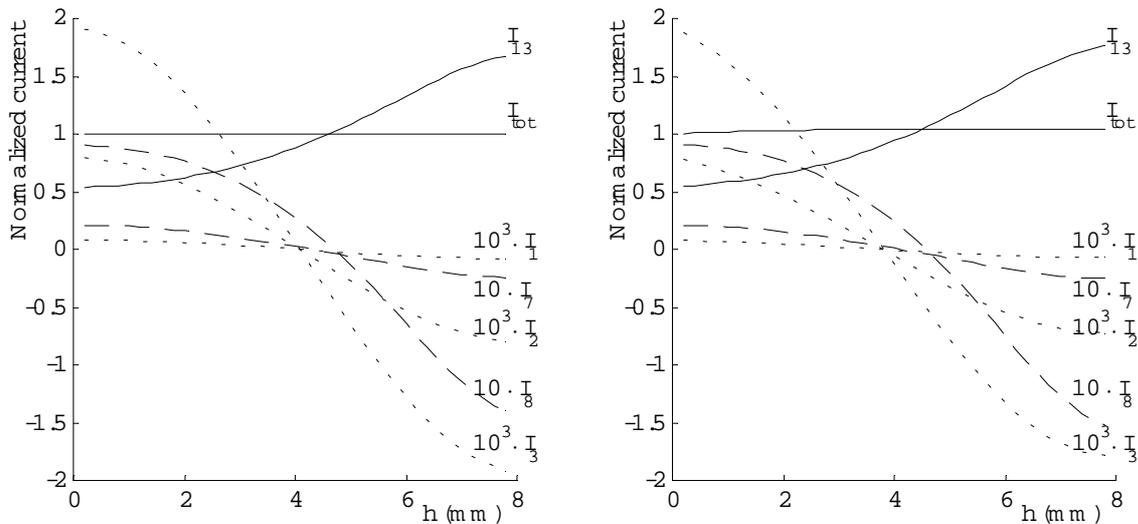
Fig. 2. Normalized currents of the electrodes when charge  $Q$  moves towards the center of the middle anode in the  $z$  direction. Here  $\gamma = 10^{-6}$  S/m (the left figure) and  $\gamma = 10^{-3}$  S/m (the right figure)
