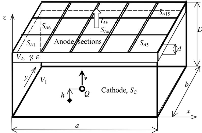
Fig. 1. An example of the resistive plate chamber
